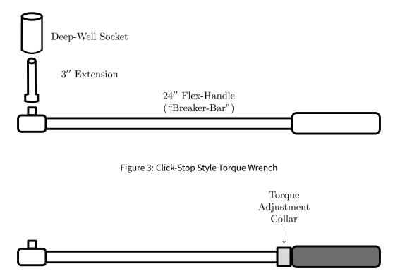
Figure 2: Flex Handle ("Breaker Bar"), Extension, Deep-Well Socket
