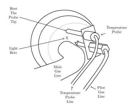
Figure 14: Lighting The Manual-Start Water Heater Pilot
