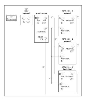
Figure 23: Pressure-Control Air Connections
