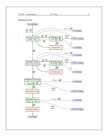
Figure 27: State-Machine Diagram
