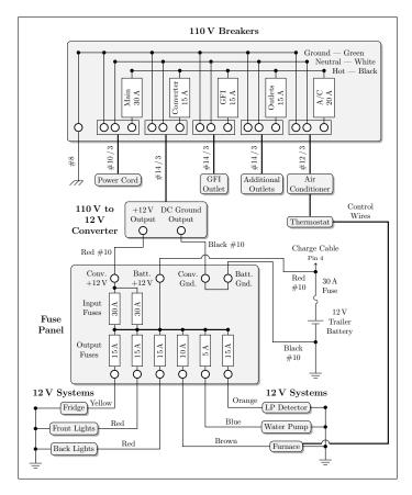
Figure 2: Wiring Diagram — Camping Trailer Electrical System
