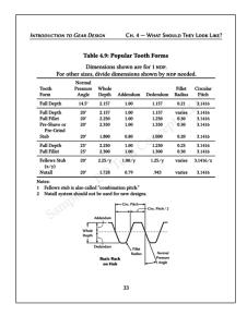
Figure 36: Gear-Tooth Forms
