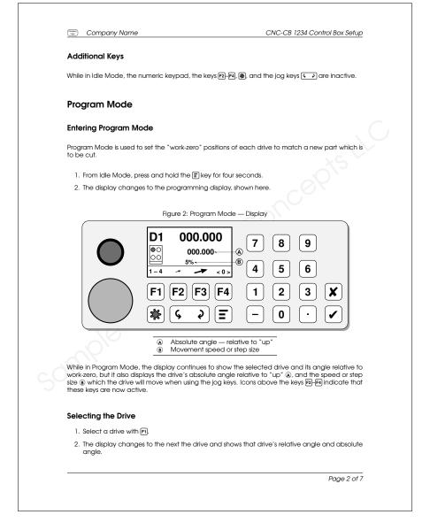
Figure 38: Front-Panel Illustration and Call-Outs
