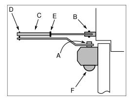
Figure 3: Parts Diagram — Automatic Door Closer — Side View
