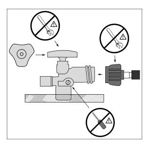
**Figure 32:** LP Tank Valve — Handle and Connection — Line Drawing
