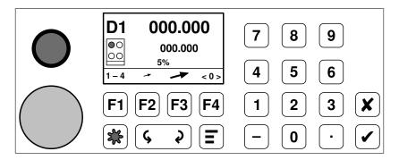
Figure 4: Control Box — Front Panel
