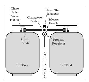
Figure 21: Diagram Label Pins — LP Gas System
